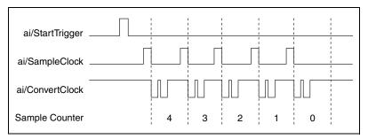
Figure 4-9. Posttriggered Data Acquisition Example
